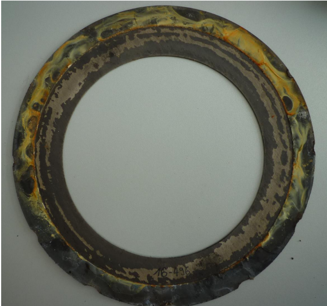
Fire test according to API 6FB (16-496)
